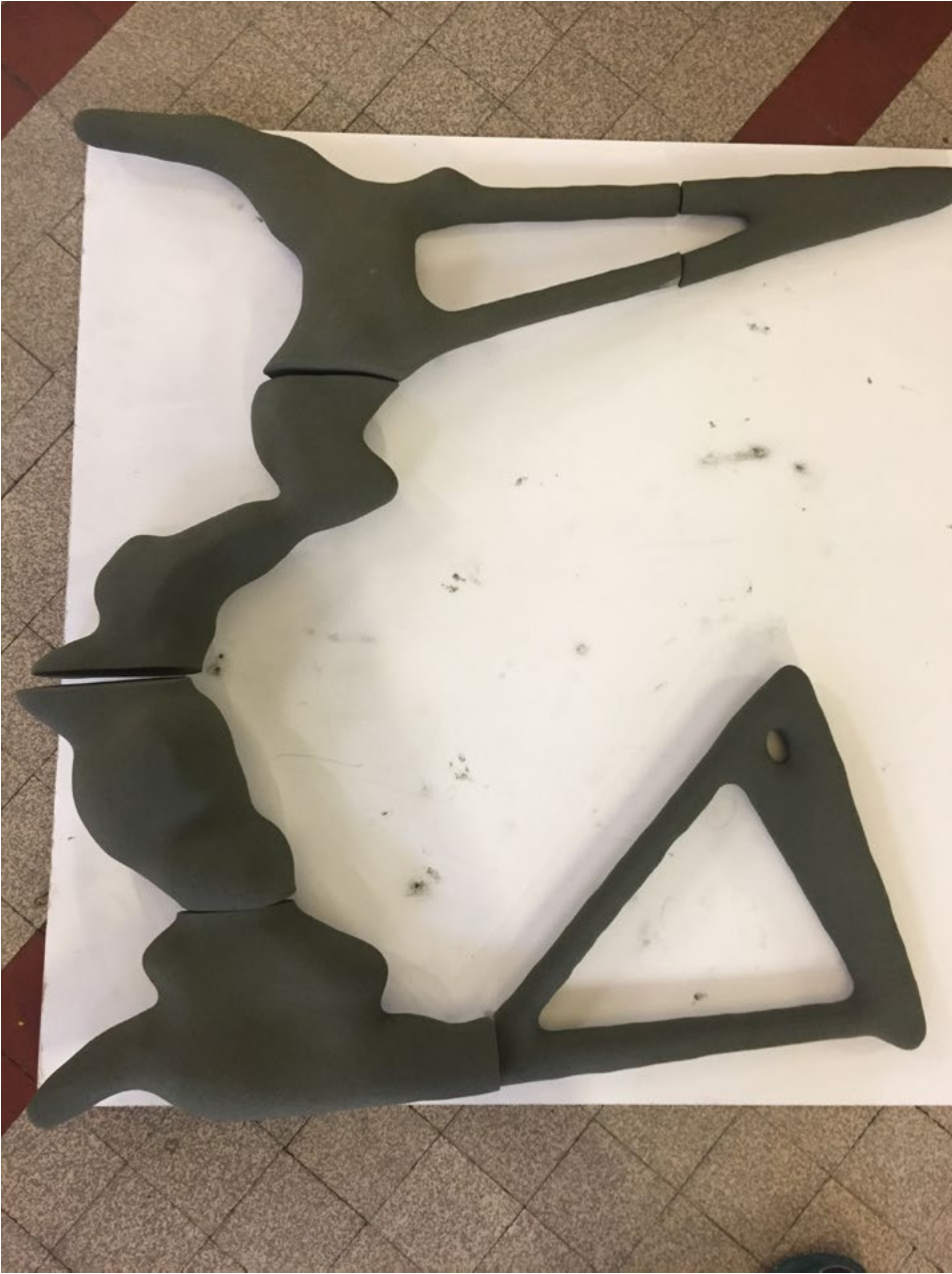
3D sand prints, in partnership with Aix en Provence ENSAM
